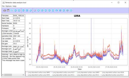
6. Please note that the agreement between SMPS-derived LDSA and Partector LDSA will depend on the size range measured by the SMPS (which depends on flow rates in the DMA and CPC). We usually get quite good agreement, in particular when the SMPS measures about the same size range as the partector 2 (10-300nm).
