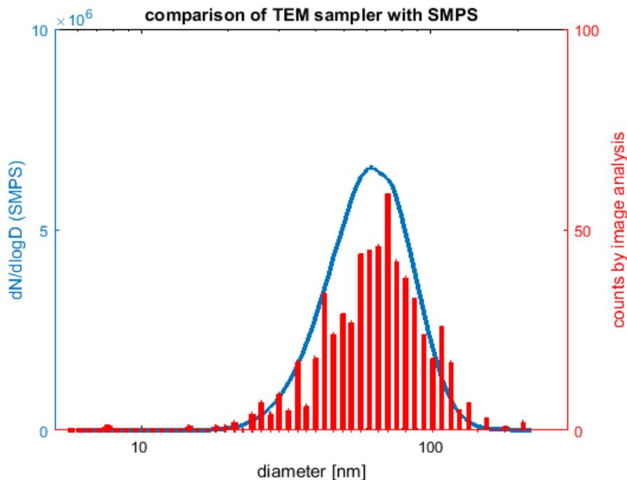
The SMPS gives a geometric mean diameter of 60.6nm, the TEM image analysis gives 63.8nm; the SMPS gives a geometric standard deviation of 1.40, the TEM image analysis gives 1.49. Despite the size dependency of the deposition, the TEM and SMPS size distribution nearly agree. Please note that all results shown here are usually for a single device, and individual devices may vary slightly in performance.
