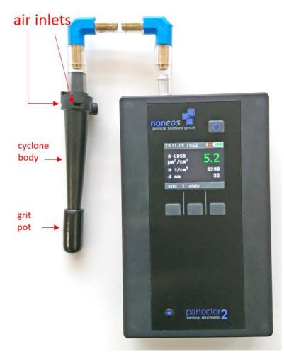
Figure 6: SKC GS-3 cyclone mounted on a Partector 2
