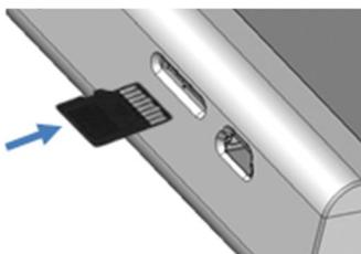
Figure 2a: Inserting the  $\mu\text{SD}$ -card
