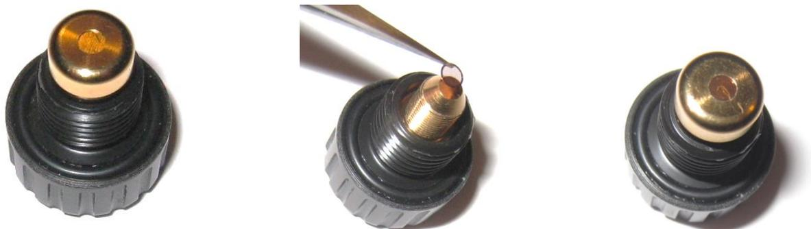
Figure 7: placing a TEM grid
