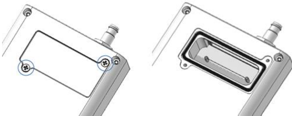
Figure 8: Charger hatch closed (left) and opened (right)
