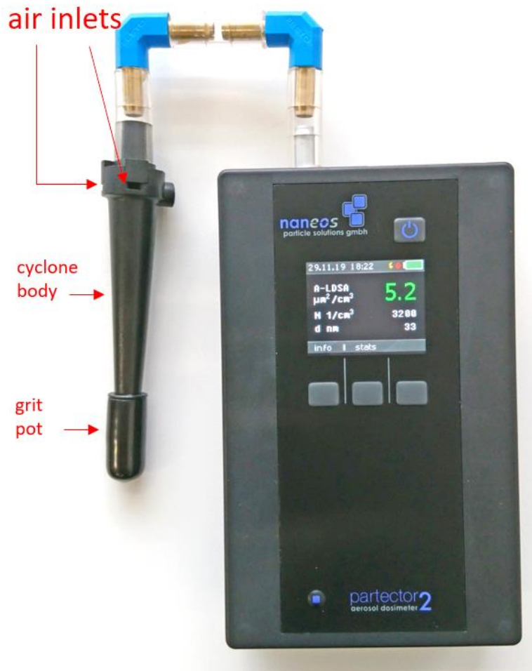
Figure 6: SKC GS-3 cyclone mounted on a Partector 2
