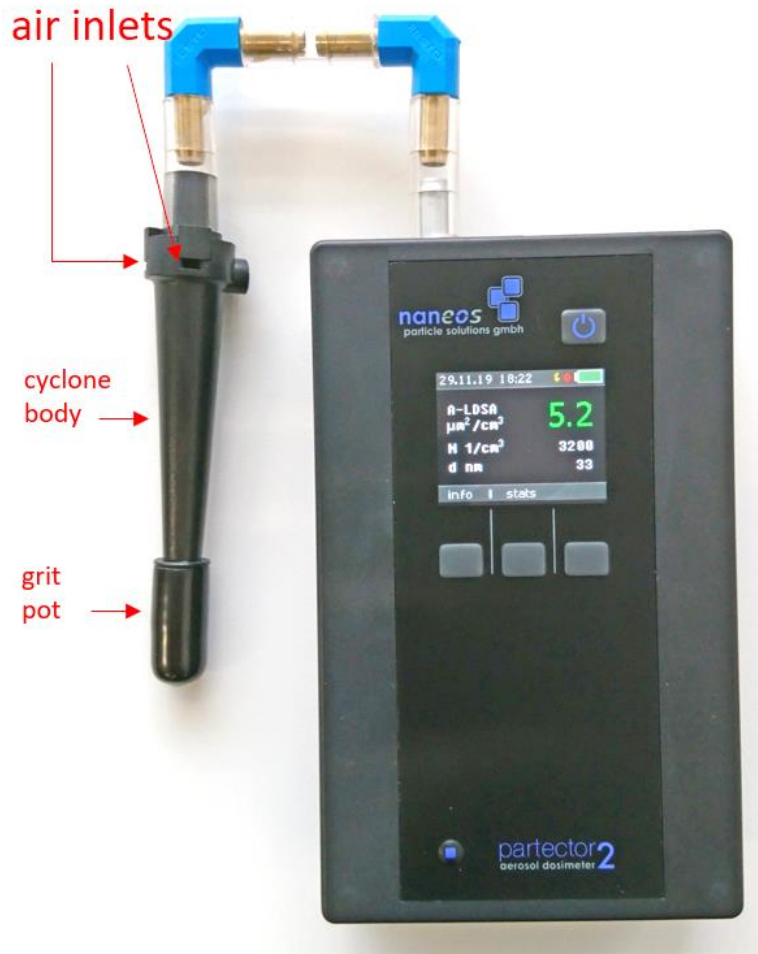
Figure 6: SKC GS-3 cyclone mounted on a Partector 2
