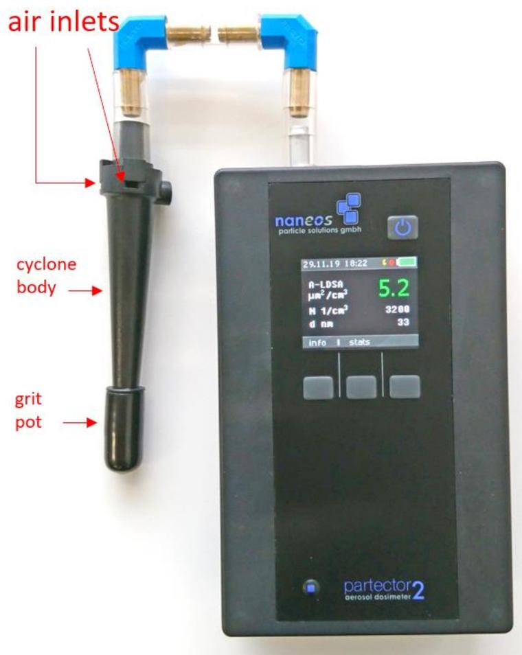
Figure 6: SKC GS-3 cyclone mounted on a Partector 2
