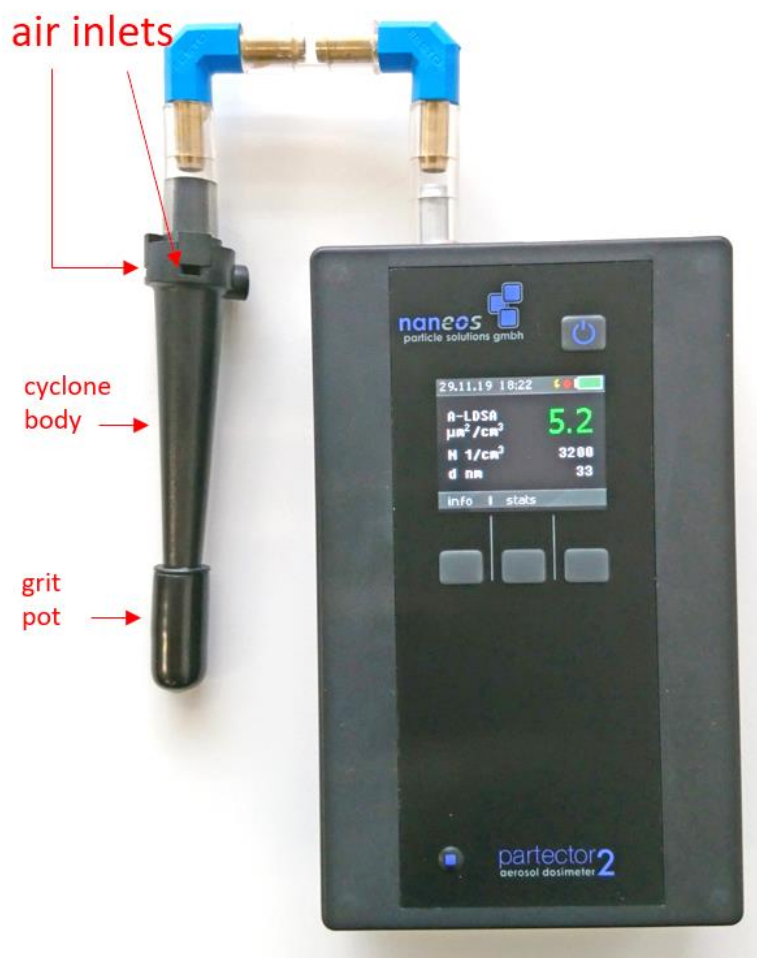
Figure 6: SKC GS-3 cyclone mounted on a Partector 2
