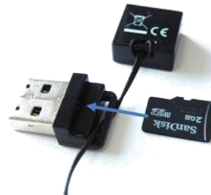
Figure 3b: Inserting the \mu SD-card into the adapter
