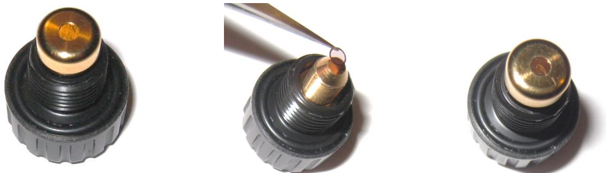
Figure 8: placing a TEM grid
